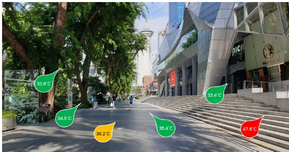
Spot readings demonstrate the cooling effect of the landscaping along Orchard Road
